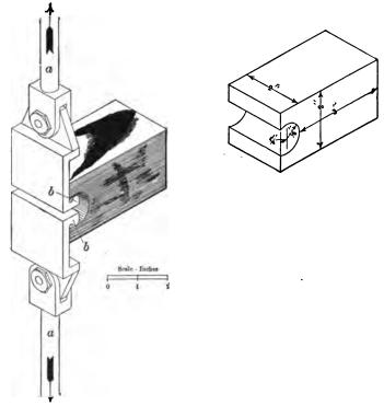
Fig. 10.—Method of making cleavability test.
